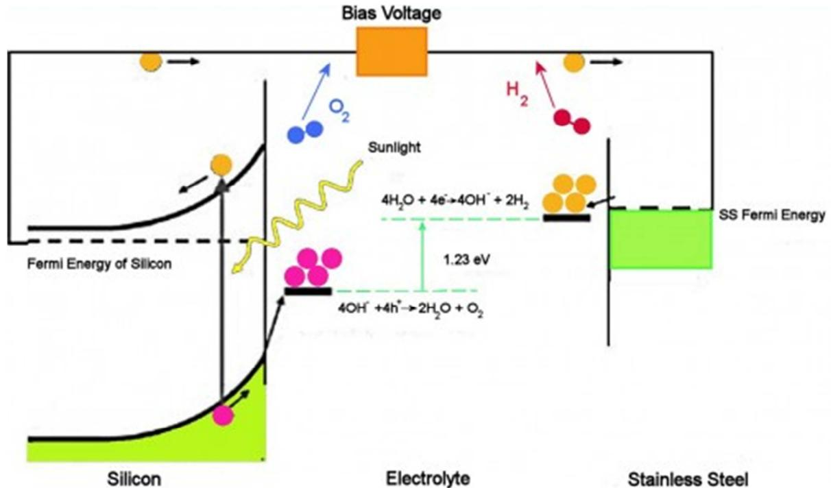
Fig. 17. The figure above illustrates how a PEC cell operates. Briefly, incoming sunlight excites free electrons near the surface of the silicon electrode.
