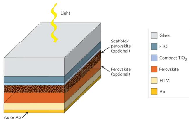
**Fig. 16.** Perovskite solar cell structure.
