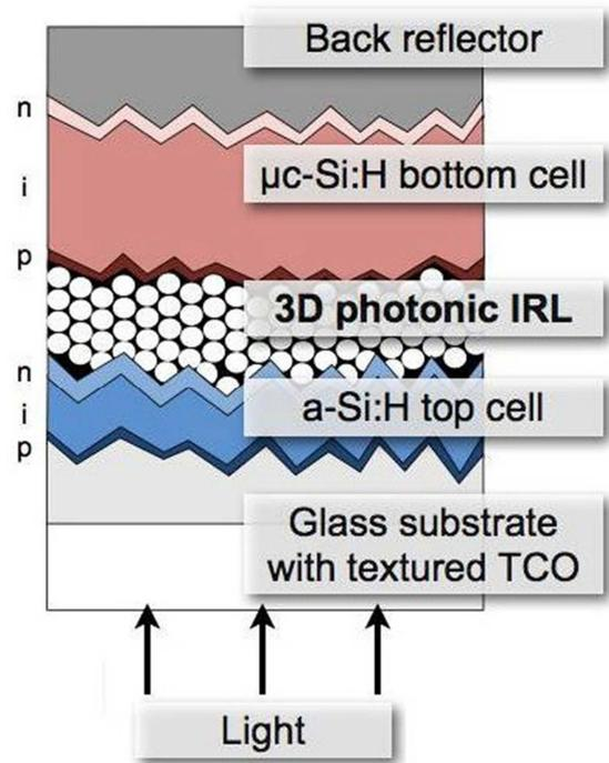
Fig. 12. Schematic structure of a micromorph silicon tandem cell with an integrated 3D photonic crystal intermediate reflector.  $\mu$ c-Si:H: Microcrystalline silicon.
