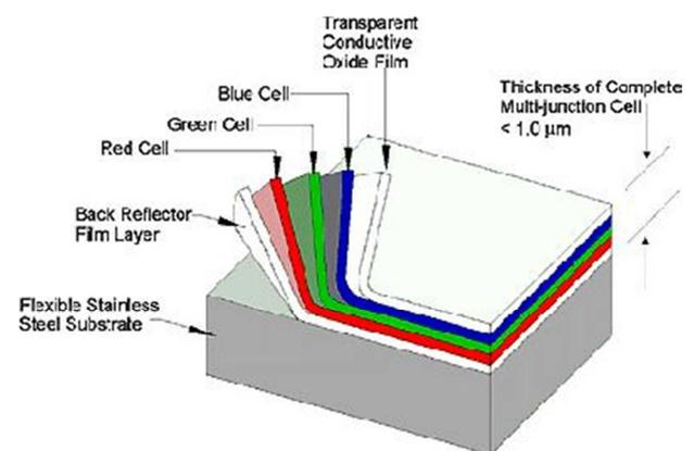
Fig. 1. Amorphous silicon is Uni-Solar. They use a triple layer system.
