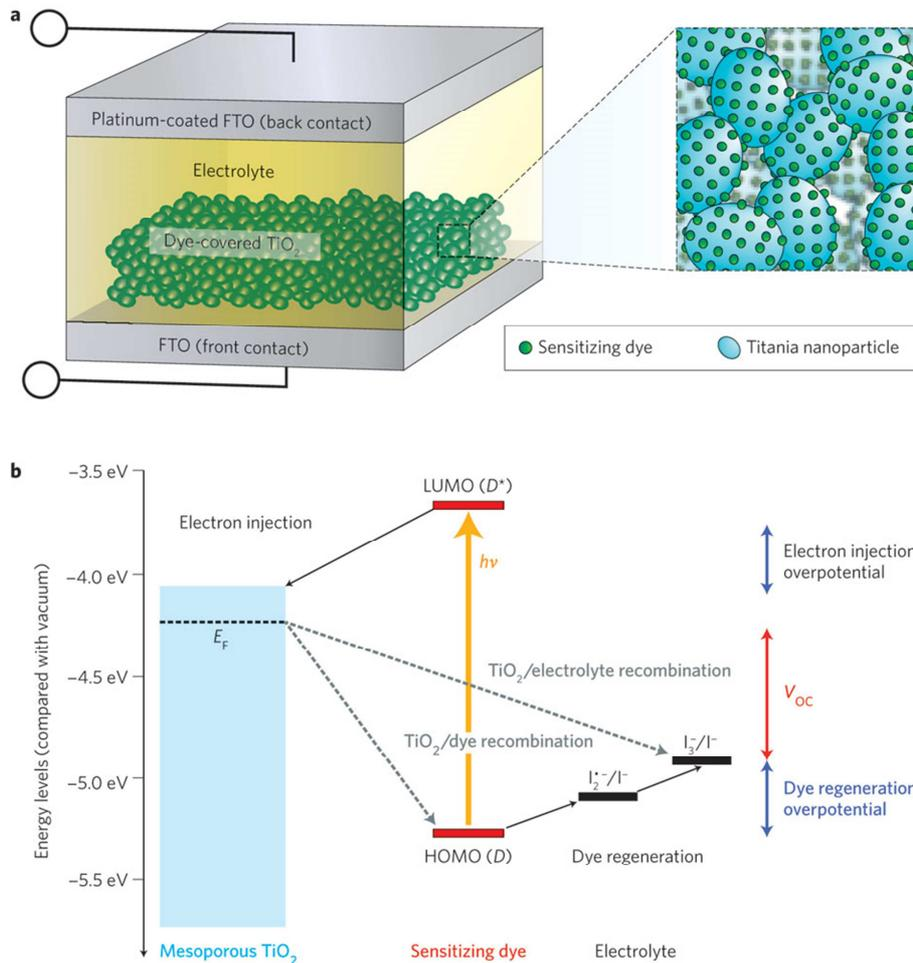
**Fig. 8.** Dye-sensitized solar cell device schematic and operation.
